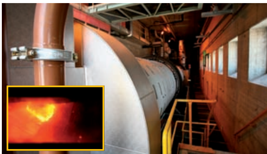
Rotary kiln for incineration of sewage sludge
