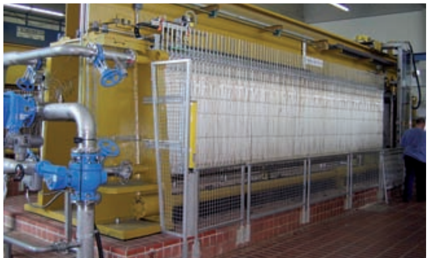
Chamber filter press with feed supply line, NP 150 / NP 40, max. 3 MPa (435 psi)
