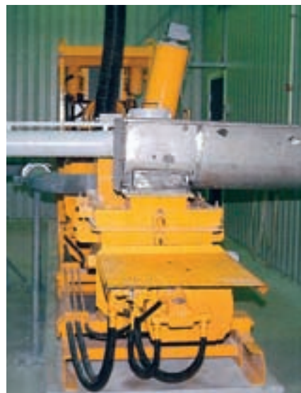
KOS 1050 sludge pump with THS 332 feeding device and hydraulic unit HA 45 on top (background). The sludge is introduced from the right and the lime from the left. One can clearly see the supported pipeline for the sludge with lime.
